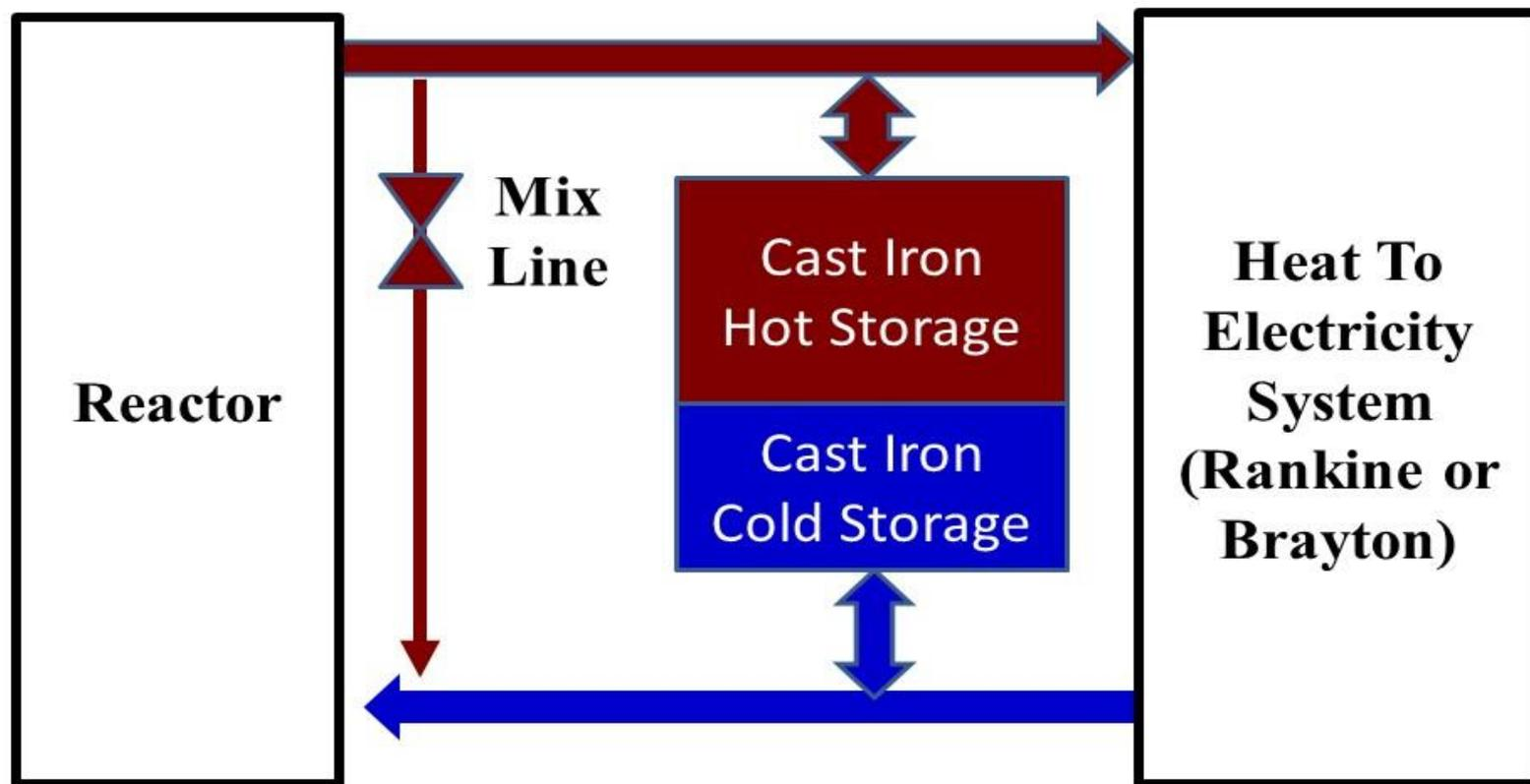
**Sodium or Salt-Cooled Reactor Intermediate Loop**
